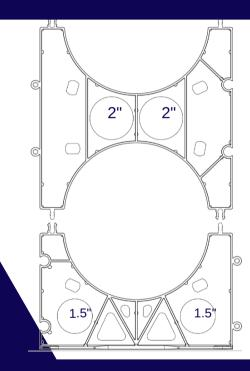
The new design includes the ability to hold 1.5" and 2" pipe within its interior.
